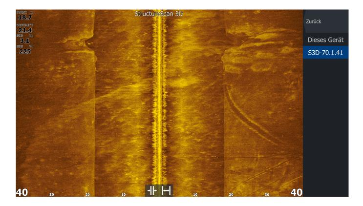
The side-scan image shows an approximately 60~m long depression on the bottom in the upper part of the image. This depression is up to 10~m wide.
